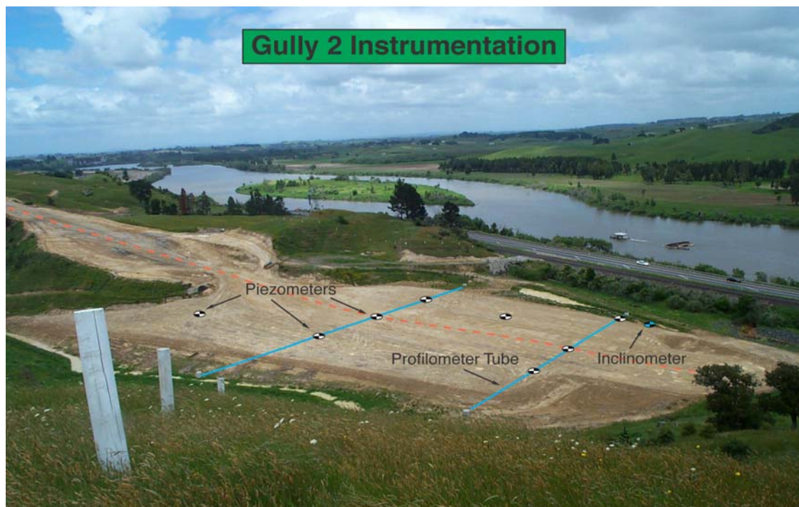
Figure 5. MLSE Gully 2 Instrumentation lines and monitoring locations.
