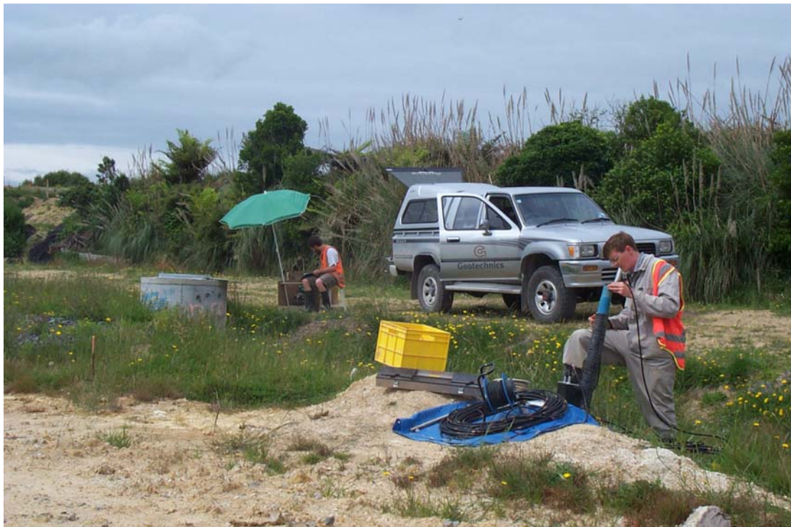
Figure 7. Monitoring of Inclinometer, Sondex and Profilometer Installations.
