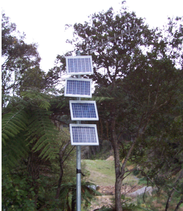
Figure 2-The 5m high steel mast at Site 2 with Solar panels and unidirectional 'Yagi' antenna mounted.
