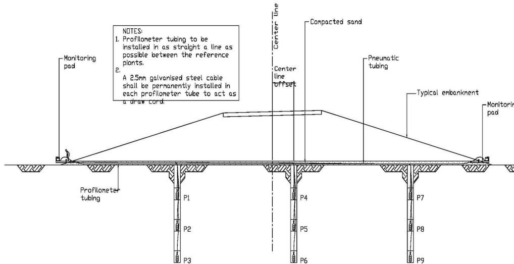
**Figure 1: Typical profilometer tubing installation beneath an embankment (including piezometer)**
