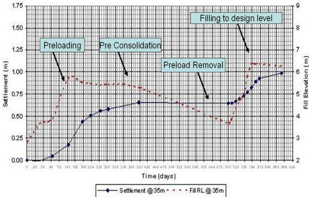
**Figure 3: Profile tube settlement versus time**
