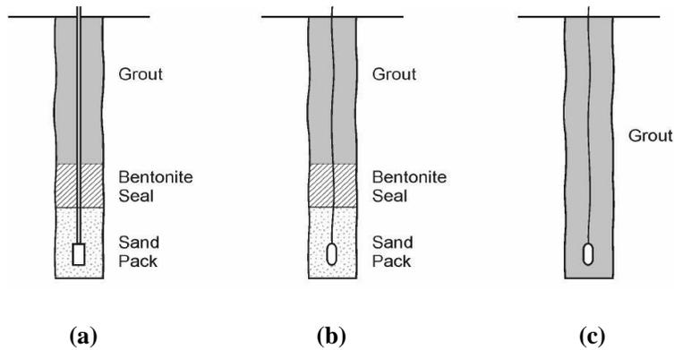
**Figure 2(a): Traditional standpipe piezometer with sand pack**
